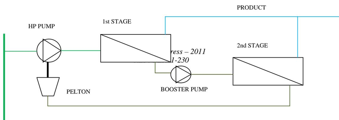
*Fig. 6. Hydraulic scheme of the racks with booster pump between stages and Pelton Wheels.*
