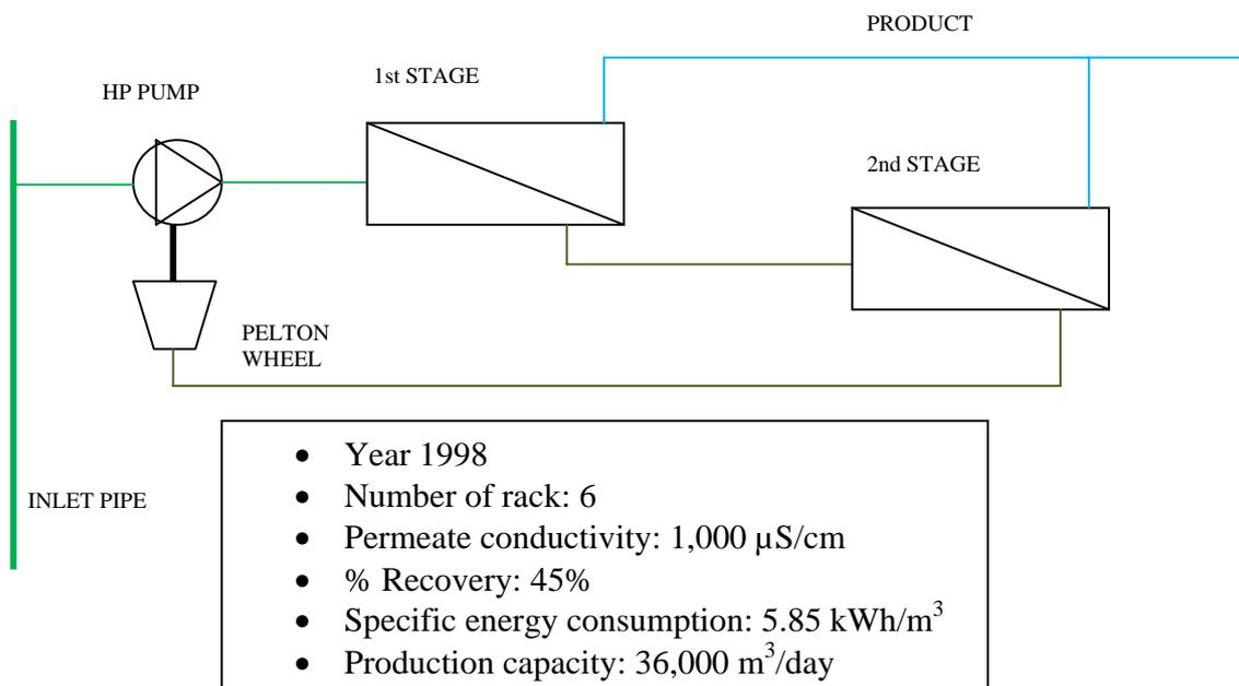
Fig. 4. Hydraulic scheme of the racks with Pelton Wheels.
