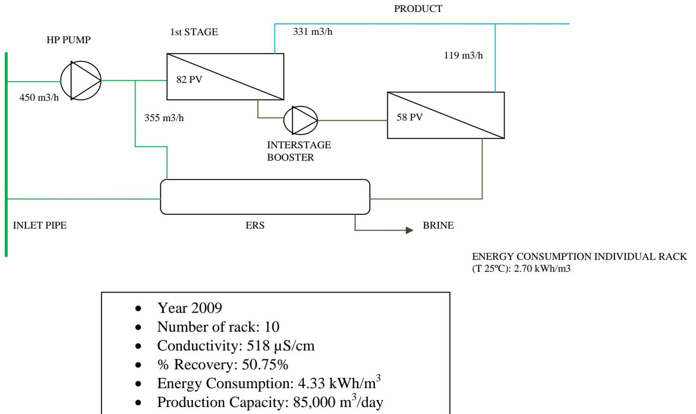
Fig. 10. Hydraulic scheme of the racks with booster pump between stages and pressure exchangers.
