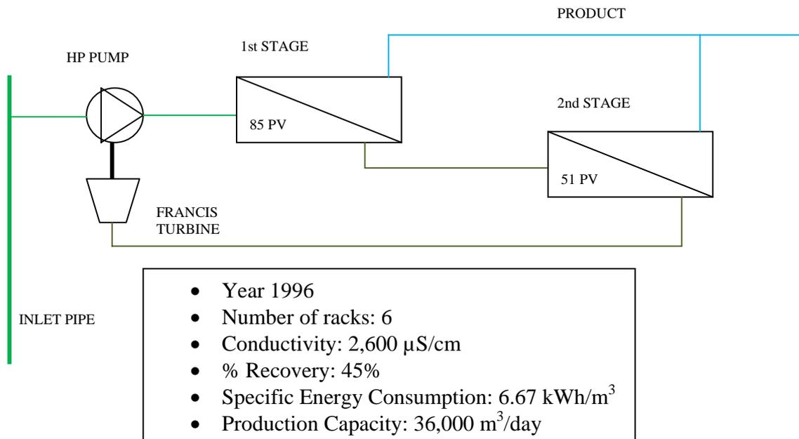
Fig. 2. Hydraulic scheme of the racks with Francis Turbines.
