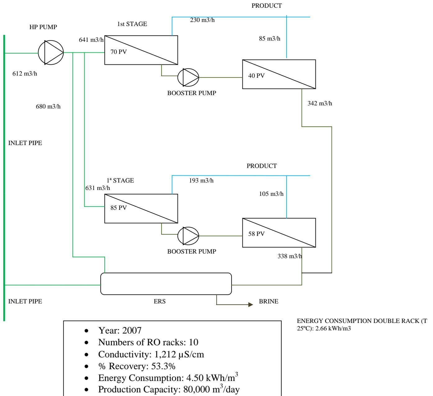
Fig. 8. Hydraulic scheme of the double racks with booster pump between stages and pressure exchangers.
